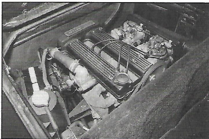
The familiar Lotus 'Big Valve' engine which could propel the Europa at over 120mph with comparative ease. Watch out for timing chain wear
