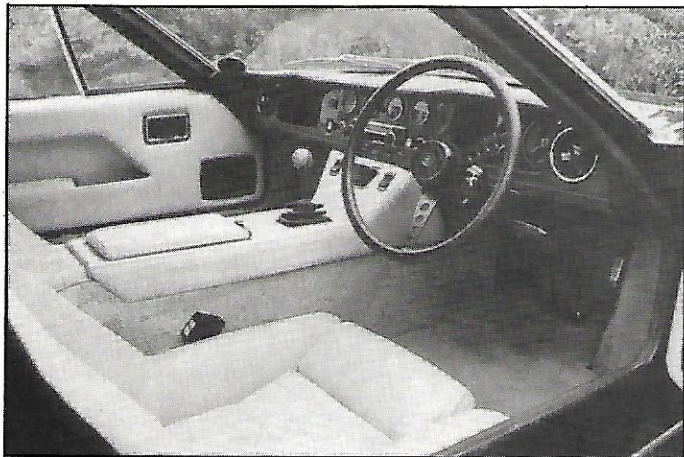
Luxurious interior of a late, five-speed Europa. Just visible under the steering wheel is the badly-positioned and rather ineffective handbrake
