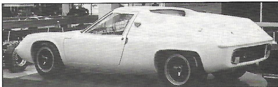
The Lotus 47 racer, above, like the Europa S1, had fixed one-piece door windows
