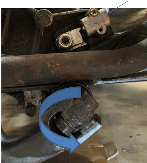
I then tightened down the rear locknut. Got in the car. Shifted through the gears. Looked like I had them! Went for a ride and low and behold, all of the gears (including 5<sup>th</sup>) and it shifts crisply and smoothly!
