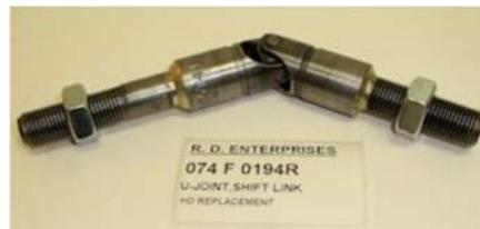
Each end of the above part is threaded to fit the proper tube. I test fit the pieces together and had about 4 1/8<sup>th</sup>, longer than the 3.75" I knew allowed the linkage to engage the gears. The end that fits in the forward tube (8) couldn't screw in all the way due to a bend in the tube, plus I needed part 15 to come up flush with the end of the forward tube (8). I took off about 1/4" of the threaded end to get it to fit.
