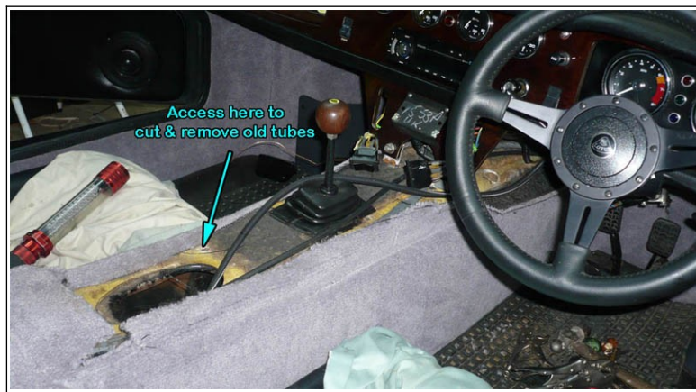
Pic 1 : Access to remove the old tubes
