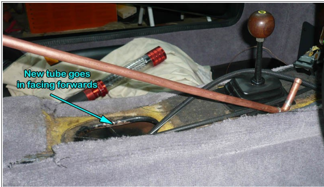
Pic 4: Tube replacement.
