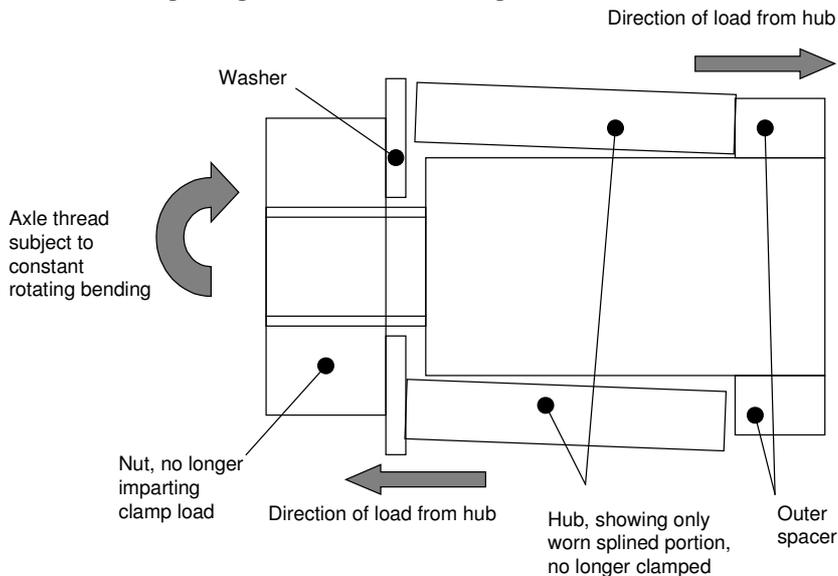
Applying Loctite to the splines stiffens the assembly and offers much greater resistance to transference of rotating bending loads along the axle, but has the disadvantage that should the clamp load drop off it will be masked. It's possible that a Loctited hub will continue to operate satisfactorily whilst inadequately clamped bearings start to create their own problems independently.
