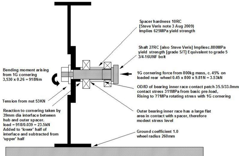
The basic tension from the hub nut tightened to 150ft-lbs translates to 311MPa surface stress at the inner bearing to spacer interface, duplicated at the inner bearing to axle face. This on its own isn't enough to cause material deformation.
