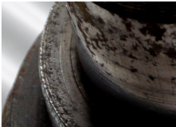
Left picture of the bearing abutment on the axle removed from the LHS of my Europa.
